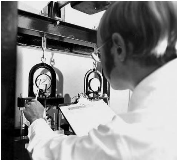
FIGURE 2.77 Reading deflection vs. time with the consolidometer.
