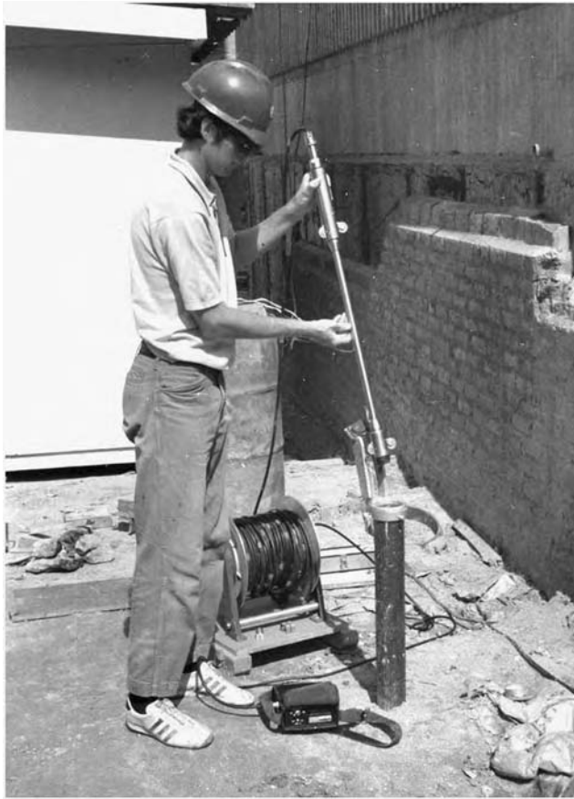
FIGURE 3.16 Slop indicator inclinometer, grooved casing, cable, and digital readout.
