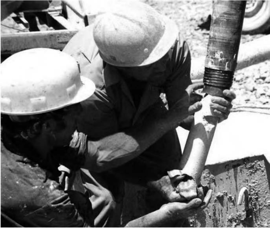
FIGURE 1.77 Removal of HX diameter limestone core from the inner barrel of a double-tube swivel-type core barrel.
