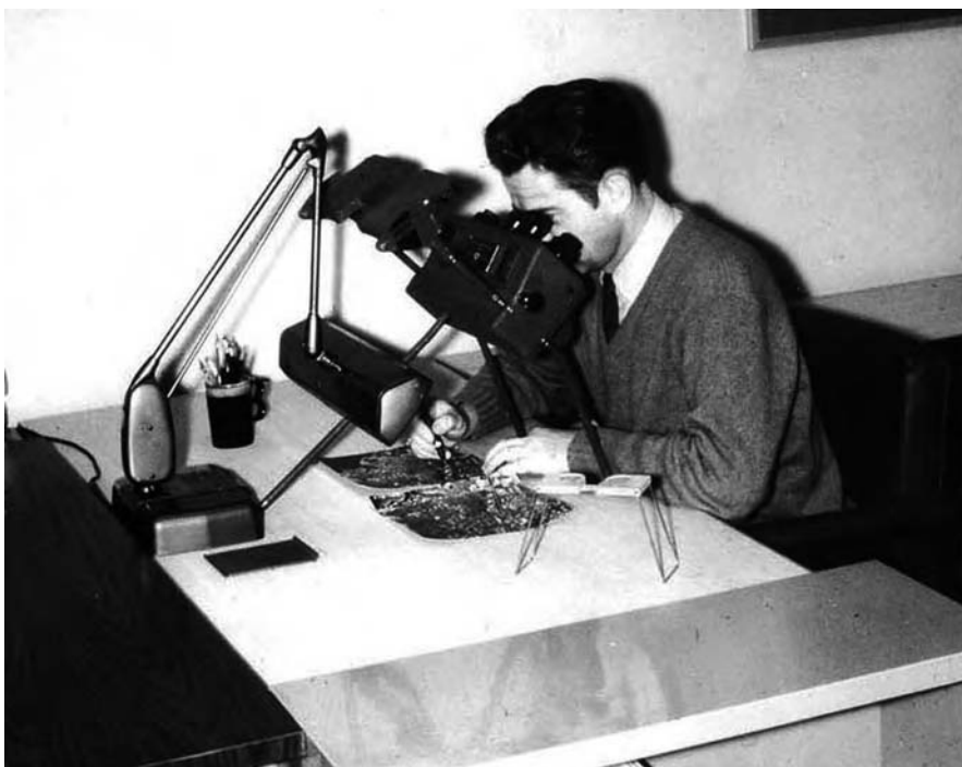
FIGURE 1.13 Stereoscopic interpretation of aerial photographs. Two types of stereo-viewers are shown.
