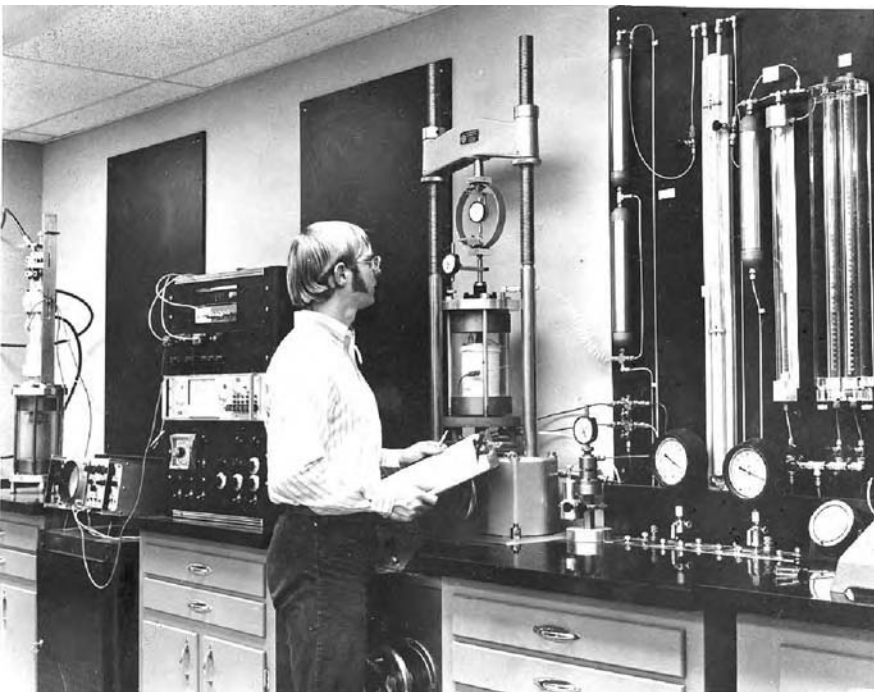
FIGURE 2.50 The triaxial compression chamber, load application, and measurement system.
