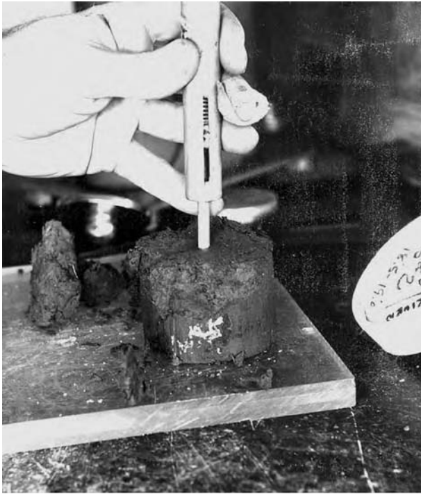
FIGURE 2.55 Pocket penetrometer applied to a Shelby tube specimen.
