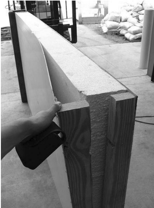
11.18 General failure mode of CSIPs (debonding followed by connection failure).
