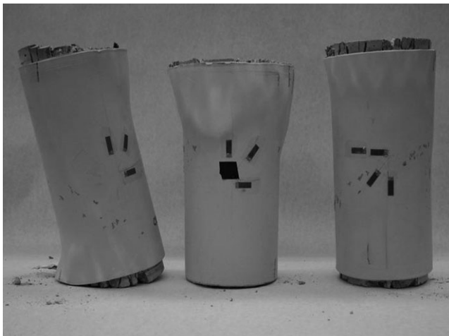
13.18 Comparison of failure among CyPB6 cylinders.
