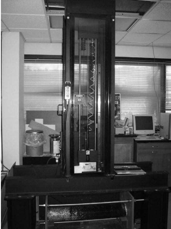
13.20 Instrumented drop weight low velocity impact test.
