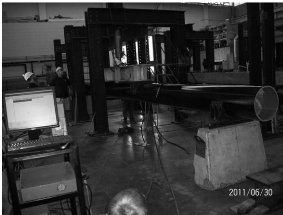
16.17 A 16 inch FRP pipe being tested at WVU-CFC Laboratory.
