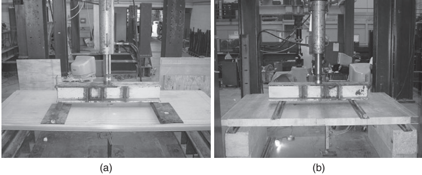
16.6 Full-scale panels under four point bend loading: (a) 4' × 10' with span 100", (b) joined panel of 4' × 5' with span 80".
