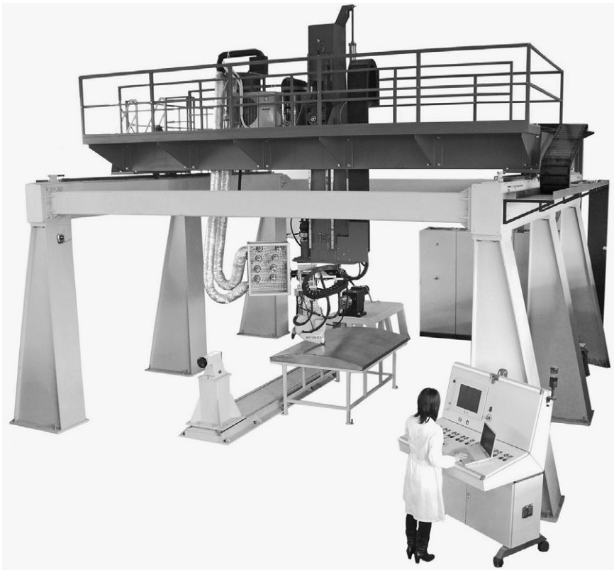
3.7 An advanced automated fiber placement machine (photo courtesy of MIKROSAM A.D. – Macedonia).
