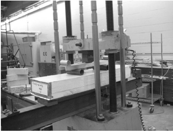
11.12 Test setup with test instrumentation ASTM C 393 (2000).
