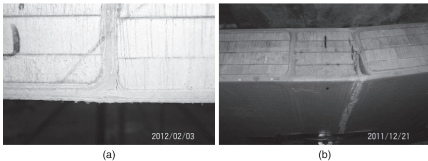
16.29 Cracking initiation and growth of a sandwich sample under three-point bending fatigue, leading to eventual failure at the corner.
