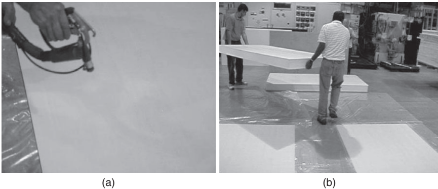
12.4 CSIP being manufactured using hot-melt impregnated spray adhesive: (a) TP spray adhesive being spread on the facesheets, (b) ready panels being stacked.
