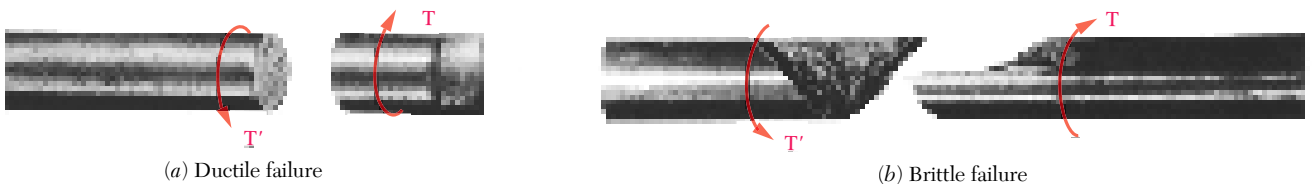
Photo 3.2 Shear failure of shaft subject to torque.
