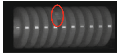
(b) Eliminating the two ends of insulator based on dilation operation
