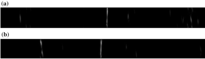
Fig. 5.27 Extraction result of slide plate cracks
