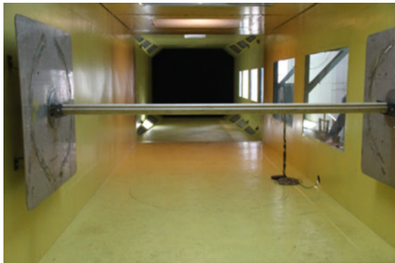
Fig. 3.8 Test device for contact line static coefficients measurement
