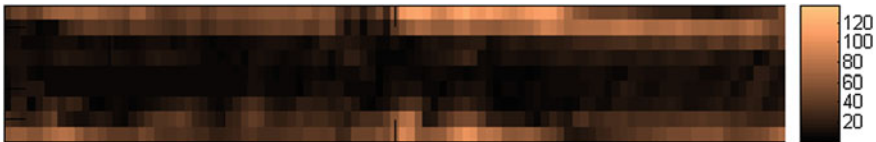
Fig. 5.13 Coefficients' distribution of slide plate edge extraction defects
