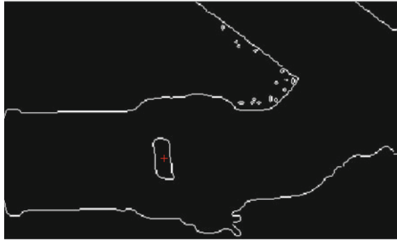
Fig. 6.59 Rectangle positioning of clevis crack
