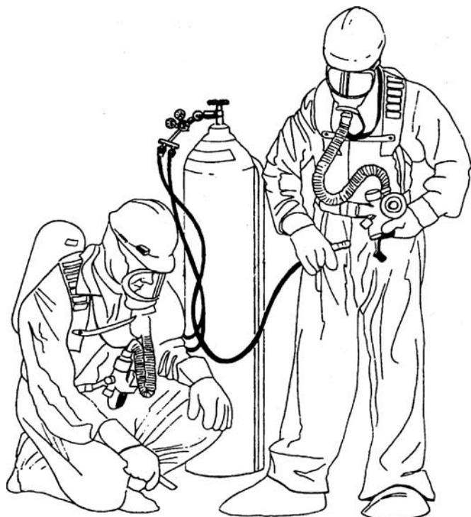
Figure 13.2. Atmosphere-supplying respirators: SCBA and supplied air shown with level B suits.
