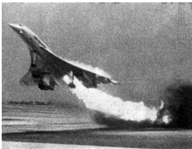
Figure 18.2. The Concorde's last flight in the year 2000. A piece of metal on the runway caused a tire explosion. Debris from the tire punctured the wing fuel tank and the fuel caught fire. Photo from Associated Press. Available at: http://www.airdisaster.com/photos/afsst/2.shtml . See color plate.
