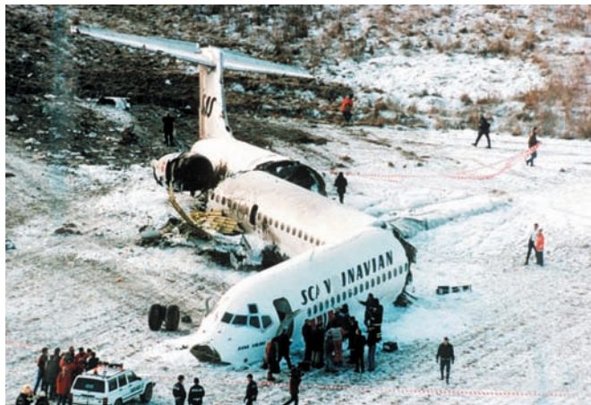
Plate 18.3. The 1991 MD-81 crash in Stockholm was caused by engine failure at low altitude when clear ice from the wings was sucked into the engines. During the emergency landing, the aircraft's momentum was reduced by hitting a number of trees before crashing on a snowy field. The snow probably prevented a postcrash fire.
