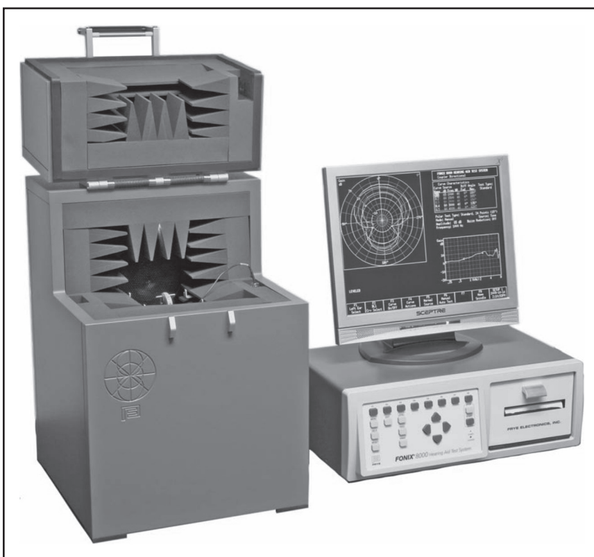
Figure 10-1. A commonly used probe microphone and hearing aid test system. The test box is on the left. Photo reprinted with permission of Frye Electronics, Inc., Tigard, OR.
