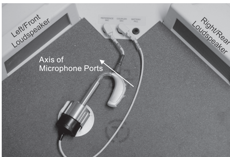
Figure 10–5. An example of the arrangement used by one probe microphone manufacturer to test the directional microphone response. From Modern Hearing Aids: Verification, Outcome Measures, and Follow-Up by Bentler, Mueller, and Ricketts. Copyright © 2016, Plural Publishing, Inc. All rights reserved. Used with permission, p. 263.
