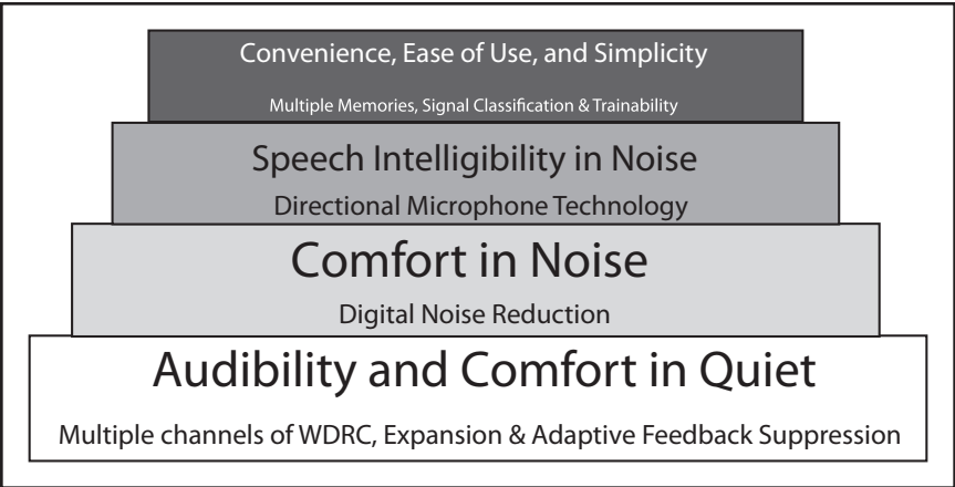
Figure 9–1. The “building blocks” of hearing aid features. For each of the four blocks, several key advanced features are listed that are designed to address it.
