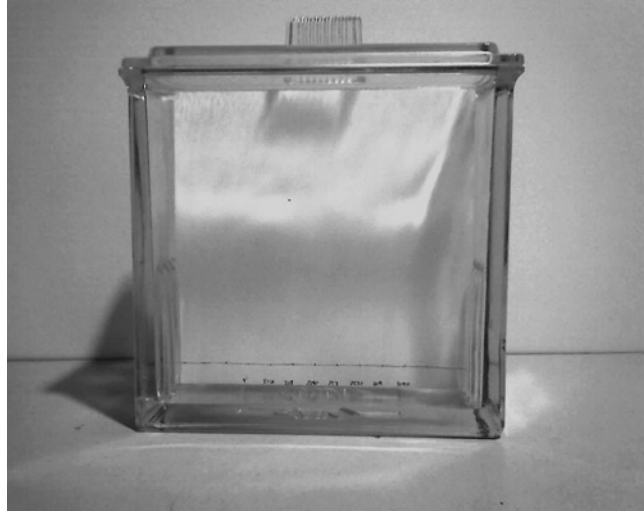
Fig. 4. TLC chromatography tank. This is an example of a TLC developing chamber able to hold and run five 20 × 20 cm TLC plates.
