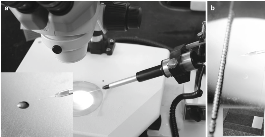
Fig. 2. Morpholino injection setup. (a) The injection setup consists of a dissecting microscope and Drummond nanoinjector. Injection solution is drawn into the injection pipette from a 3–4- \mu L drop placed on top of parafilm (a, inset). A 3 \times 1-in. microscope slide is placed on top of a larger 3 \times 2-in. slide to create a groove, where one- to two-cell-stage embryos will be positioned (b, inset). The embryos are placed with a plastic pipette and the excess fluid is removed. The embryos are lined up using pulled glass probe and much of the remaining fluid is drawn out by capillary force (can be done with a corner of a paper napkin) to leave just enough medium to prevent embryo dehydration. The embryos are injected with 4.6 nL of morpholino solution (b).
