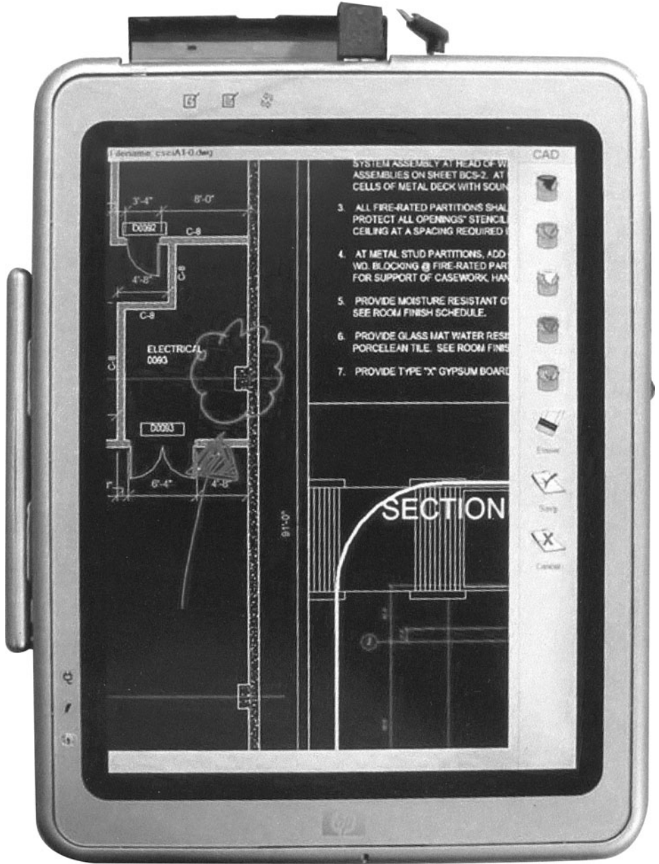
Figure 13.2 Field2Base Tablet PC transmitting portion of contract drawing to architect/engineer with questions about electrical room's wall construction. (By permission: Field2Base, Morrisville, N.C.)
