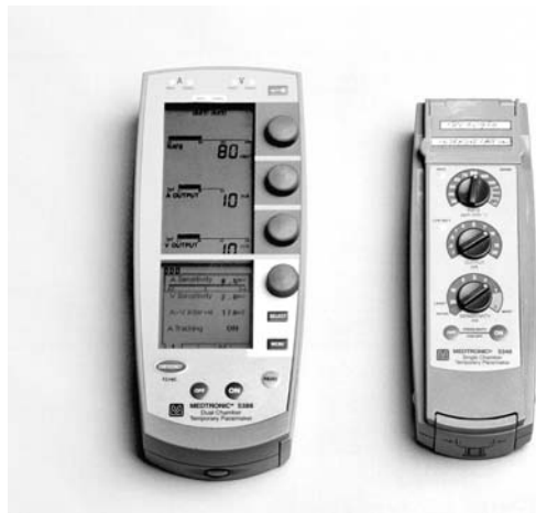
Figure 19.11 External pacemakers. Medtronic, Inc. (i) Model 5388 (dual-chamber); (ii) model 5348 (single-chamber). Both are capable of rapid pacing for certain tachycardias (see text).
