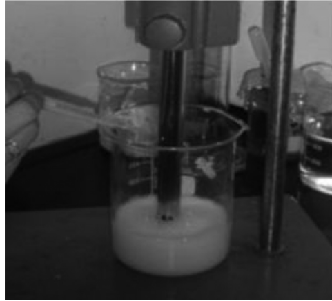
Figure 21.1. Homogenization of aqueous and organic phase using high performance disperser Ultra Turrax ® T25 with 18G mixing shaft.
