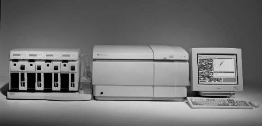
Figure 13.4 The GeneChip® Instrument System. From left to right, the hybridisation station, scanner and workstation. Image courtesy of Affymetrix. A colour version of this figure appears in the colour plate section
