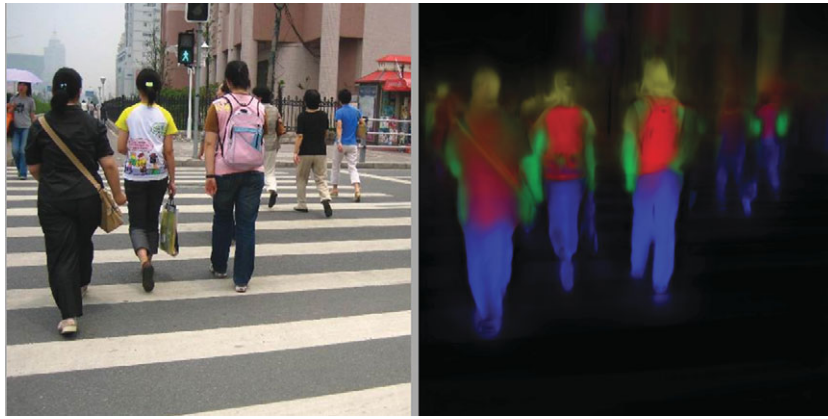
Figure 6. Just like we can learn filters for objects, we can also learn them for body parts, legs, arms, heads, torsos and hands. On the left is the image; on the right is the output of filters for body parts denoted in different colours.
