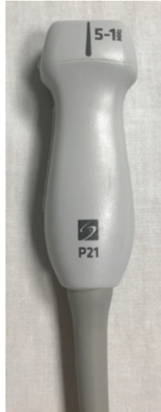
FIGURE I.11 Phased array transducer: Phased array transducers have smaller flat footprints and exhibit a pie-shaped field of view
