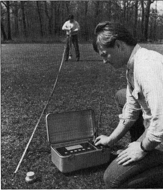
FIGURE 2.2 Portable refraction seismograph. (Courtesy of Soiltest, Inc.)
