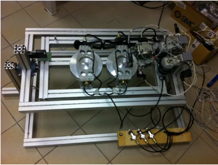
Fig. 1 The prototype of stabilized platform
