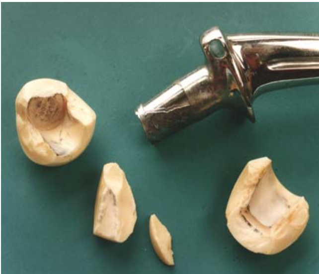
Fig. 1 In vivo destructed ceramic heads
