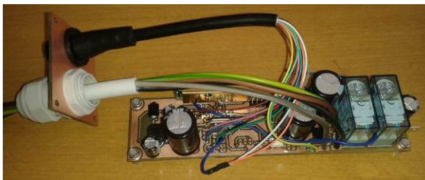
Fig. 8 Control and Power Electronics Board
