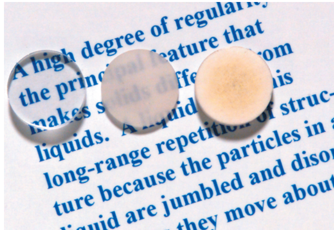
Figure 1.2 Photograph of three thin disk specimens of aluminum oxide, which have been placed over a printed page in order to demonstrate their differences in light-transmittance characteristics. The disk on the left is transparent (that is, virtually all light that is reflected from the page passes through it), whereas the one in the center is translucent (meaning that some of this reflected light is transmitted through the disk). And, the disk on the right is opaque—i.e., none of the light passes through it. These differences in optical properties are a consequence of differences in structure of these materials, which have resulted from the way the materials were processed. (Specimen preparation, P. A. Lessing; photography by S. Tanner.)
