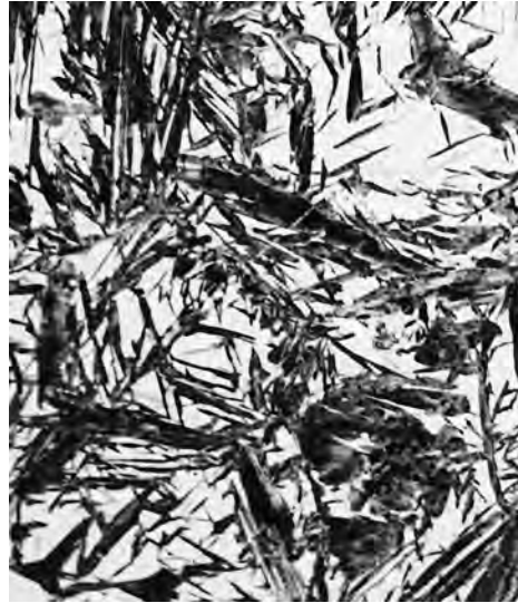
Figure 10.21 Photomicrograph showing the martensitic microstructure. The needle-shaped grains are the martensite phase, and the white regions are austenite that failed to transform during the rapid quench. 1220 \times . (Photomicrograph courtesy of United States Steel Corporation.)
