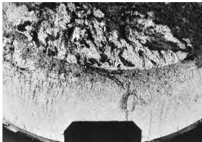
Figure 22.13 Optical micrograph of failed section of axle that shows the keyway (bottom), as well as the flat outer perimeter and rough core regions. [Reproduced with permission from Handbook of Case Studies in Failure Analysis, Vol. 1 (1992), ASM International, Materials Park, OH, 44073-0002.]
