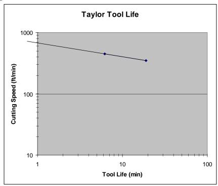
C is read from the Y-intercept and is approximately 680 ft/min. The slope, n, can be determined by taking the ln of the x and y coordinates of any 2 points and determining  $\Delta Y/\Delta X$ . It is positive because the Taylor tool life equation is derived assuming the slope is negative. Using the points (1,680) and (19,350) the slope is about 0.226.
