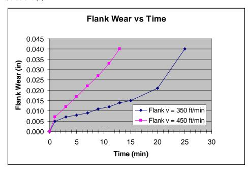
Using the graph, at 350 ft/min the tool last about 6.2 min; at 450 ft/min, it lasts 19.0 min.
