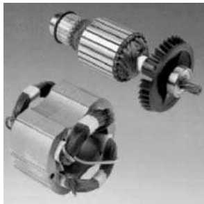
Figure 9.6 The main components of a d.c. machine. (Source: www.csd.ijs.si/applications/doptimel/Euromicro2001.pdf ).
