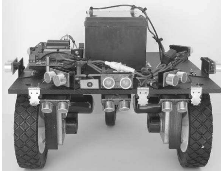
Figure 8.17 A robotic base showing sensor positions. (Courtesy of The Open Automation Project.)
