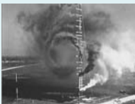
V3.5 Aircraft wing tip vortex
