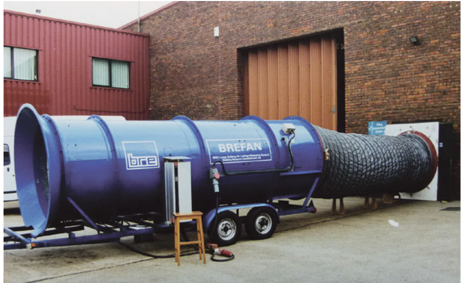
Figure 11.11 Testing for whole building airtightness
