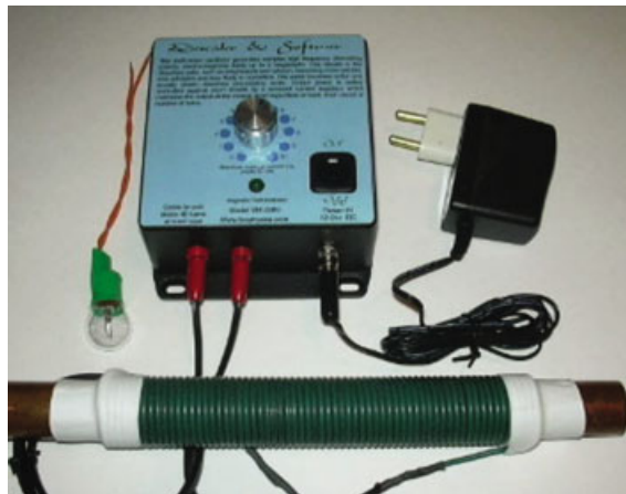
Figure 1.1 Water 'treatment' magnets and 'electronic descaler' – might as well be an ornament
