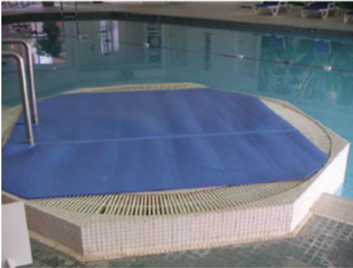
Comparative before and after to show quick effect of covering a spa area to conserve evaporation and heat. A purpose-made close-fitting cover would show better results.
