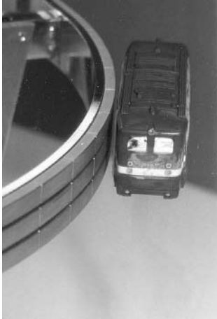
Figure 11.41 Contactless superconducting levitated model train gliding at the side of the track [11.68]
