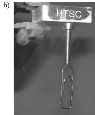
indicated in Figure 10.6. b Technical proof of the magnetization state of the HTSC bulk based on the evidence of magnetic forces on iron parts (a screw and a paper clip hanging on the SPM)
