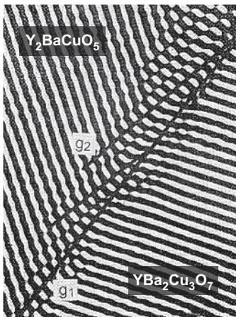
Figure 2.21 Sequence of planar defects at the interface between 123 matrix and 211 grain (Fourier filtered TEM) [2.49]
