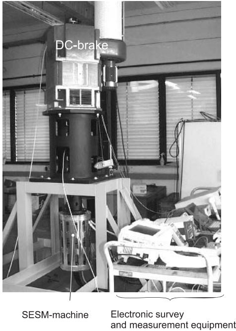
Figure 12.12 Test bench for high-dynamic SESM equipped with load machine (DC brake), feeding and survey equipment [12.25]
