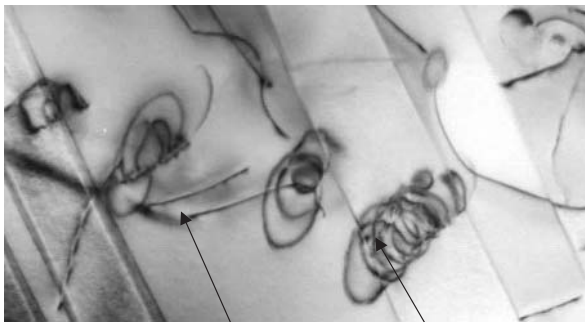
Full and partial screw dislocations (generated under strain in 45^\circ to (001))
