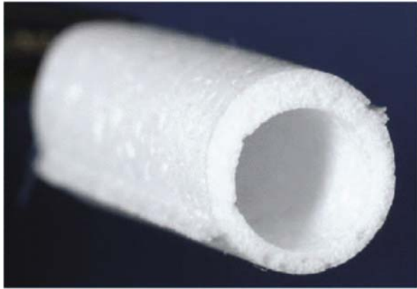
Fig. 7.3 Example of a biodegradable scaffold for vascular tissue engineering (Schmidt D et al. Ann Thorac Surg 2004)
