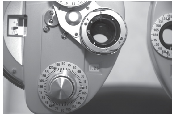
Fig. 4.12 The Jackson cross-cylinder (JCC) on a phoropter. The JCC is set up to assess the correcting cylinder axis.
