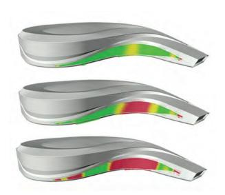
Figure 1.32: Thornton Tomasetti's CORE studio assisted 360 architects in the panelization of the Rogers Place Arena in Edmonton, Canada. A bottom-up approach was used to derive panel layout controlled by physics engine Kangaroo for Grasshopper. © *Thornton Tomasetti CORE studio*
