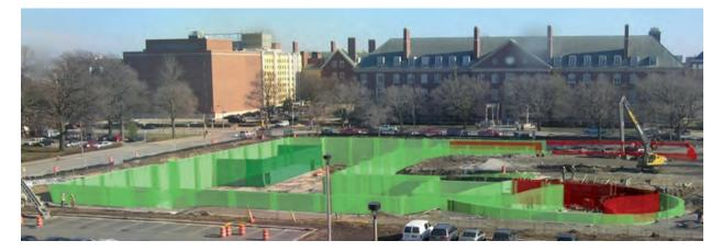
Figure 7.3: Visualization of construction progress deviations: BIM elements superimposed over a time-lapse image, color-coded based on their progress deviations. Elements behind schedule are color-coded in red, on schedule colored in green. © *MGF*
