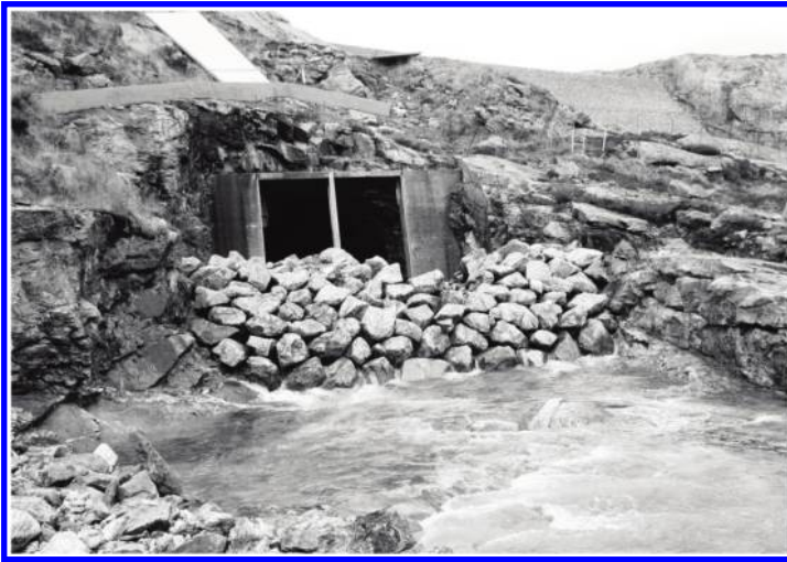
Figure 2. Test site in the outlet channel of the spillway of the Svartevatn dam in Norway. Test dam 3 in 2012 which did not fail completely in the front and the 129 m high Svartevatn dam in the background.
