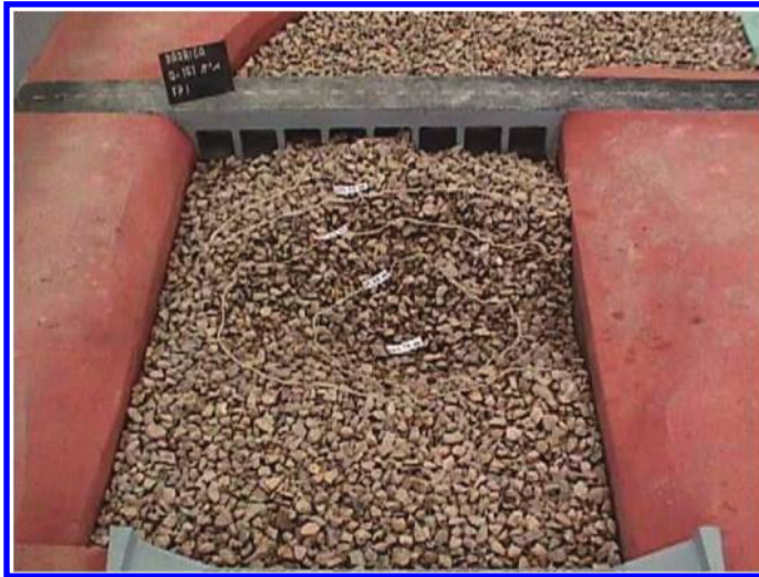
Figure 12. Erosion in the mobile bed model of the plunge pool performed at the LNEC.
