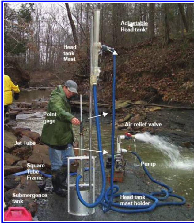
Figure 21. Jet Erosion Test performed in situ (picture from USDA-ARS).
