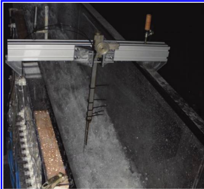
Figure 7. Installation of equipment for two-phase flow local measurements in testing channel.
