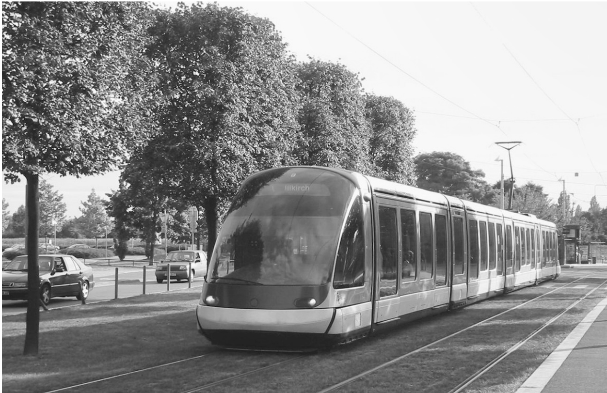
FIGURE 12-27 In Strasbourg, Germany, the right-of-way for the tramway is grass, helping give the city a greener visual appearance. Image acquired from depositphotos.com.
