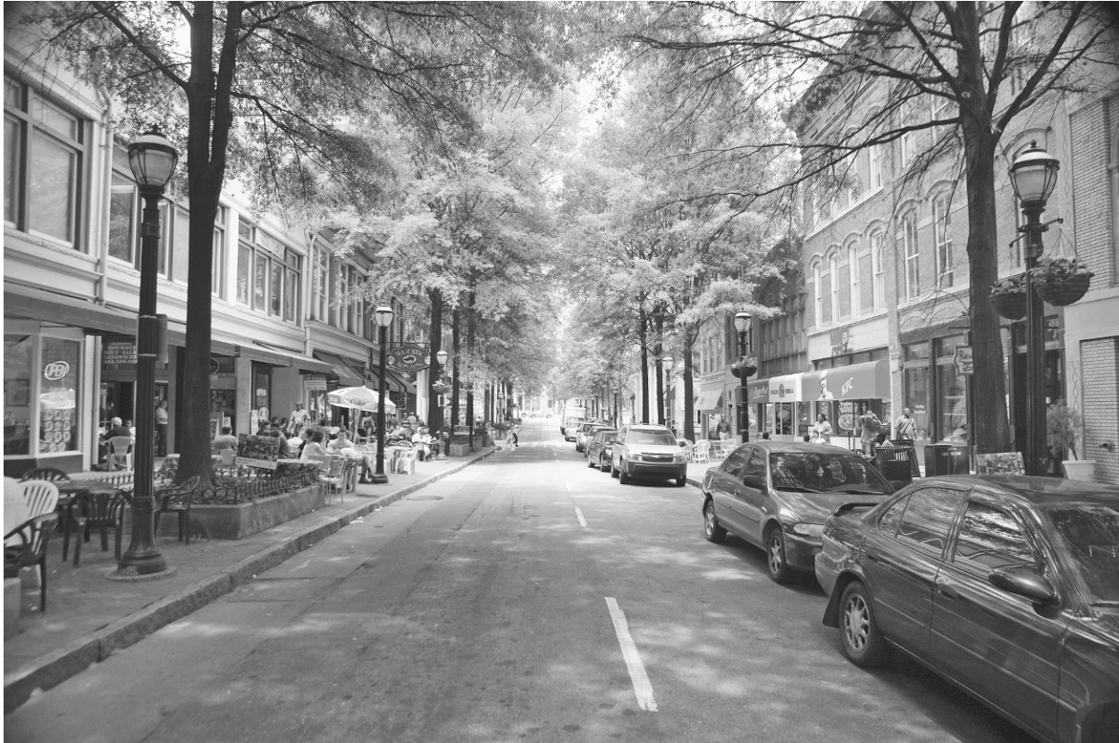
FIGURE 3-17 The combination of narrower streets, on-street parking, and wider pedestrian spaces slows down traffic and creates a more pedestrian-friendly corridor along Atlanta's 15th Street. Image courtesy of EDAW.
