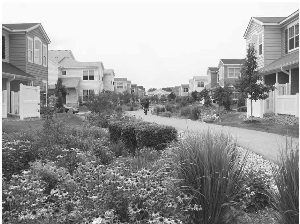
FIGURE 7-12 A rain garden can be placed almost anywhere, but is most useful if positioned to collect runoff, such as near a driveway, road, or sidewalk, or at the base of a slope. Image courtesy of Jamie Csizmadia.
