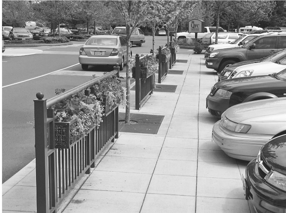
FIGURE 6-5 In Seattle, Washington, metal railings help create a sense of separation from the road, and are also used to hold up decorative planters. Image courtesy of www.pedbikeimages.org / Dan Burden.
