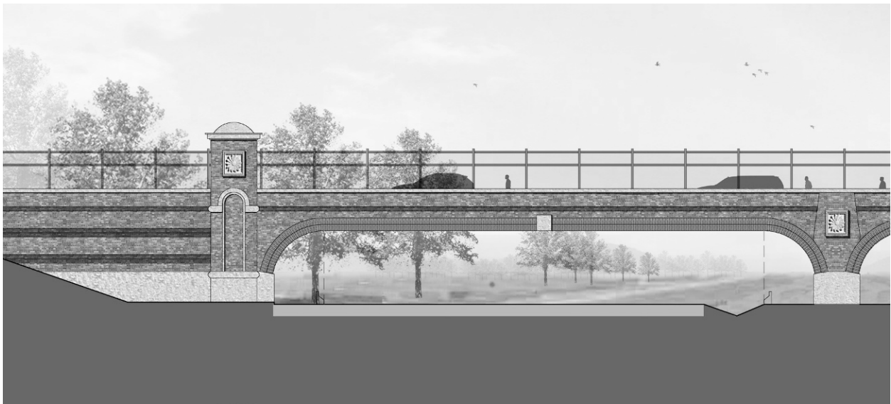
FIGURE 4-3 Various concepts were explored for the bridges of the Monroe Connector/Bypass. Major bridges showed a feature called a freestanding pylon that is reminiscent of a clock tower. Image courtesy of AECOM.
