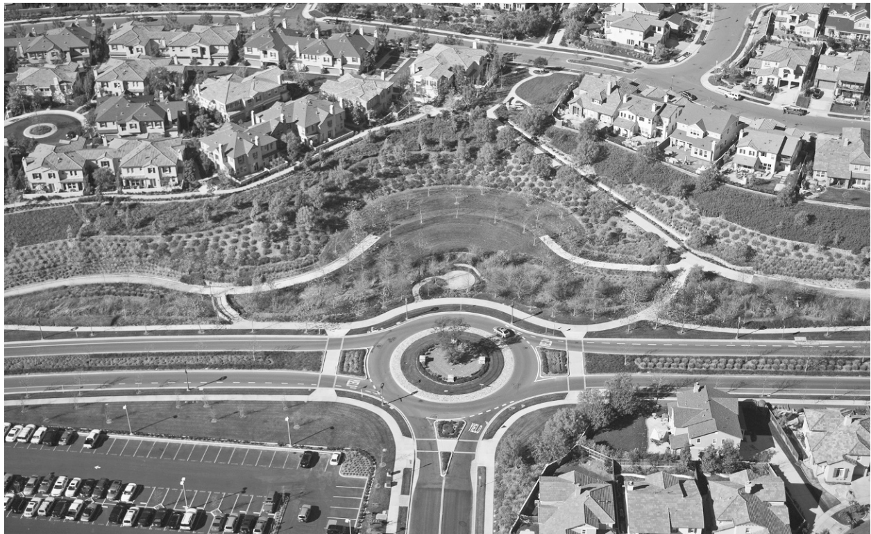
FIGURE 7-9 Ladera Ranch has several green features, such as roundabouts at small intersections, narrow street widths, and landscaped medians. Image courtesy of AECOM.
