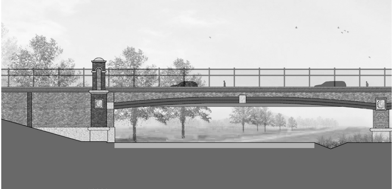
FIGURE 4-2 The Monroe Connector/Bypass is toll road along a twenty-one-mile corridor in central North Carolina. Aesthetics were a major consideration, with the overall theme being based upon a combination of brick and stone surfaces to give the roadway's bridges a classic look. Image courtesy of AECOM.
