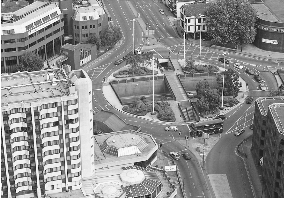
FIGURE 3-16 The Old Market Roundabout in Bristol, England, has traffic lights at every entrance (not typical for roundabouts), a road that passes beneath it, and gardens in the center. Image courtesy of Wikipedia Commons.
