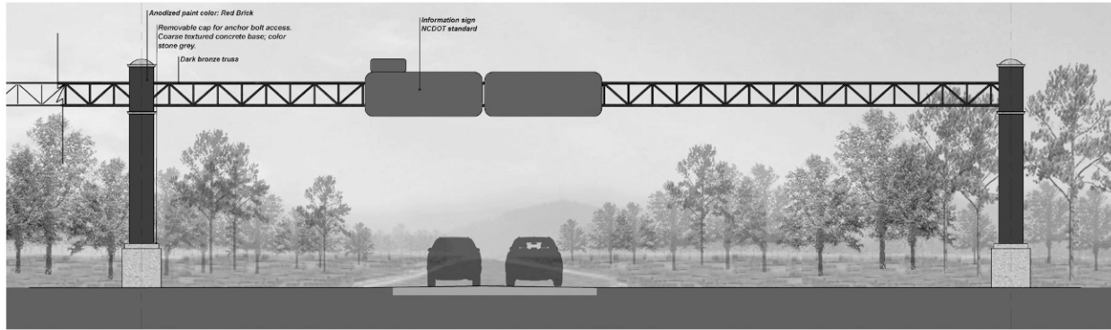
FIGURE 11-1 The Monroe (North Carolina) Bypass was designed as a single contiguous toll project, meaning that instead of toll booths, the project includes using electronic transponders and cameras so motorists will be able to drive without ever having to stop to pay a toll. Image courtesy of AECOM.
