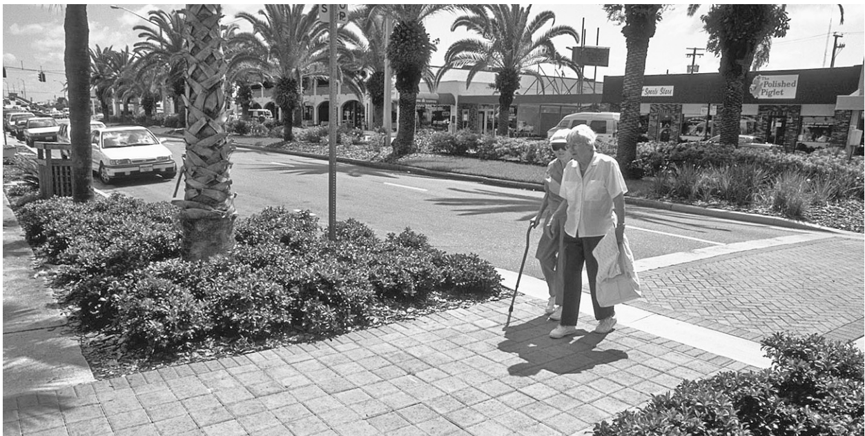
FIGURE 3-7 Pedestrians in Venice, Florida, are using a curb extension that improves the visibility of pedestrians and reduces their exposure to motor vehicles. Image courtesy of www.pedbikeimages.org / Dan Burden.
