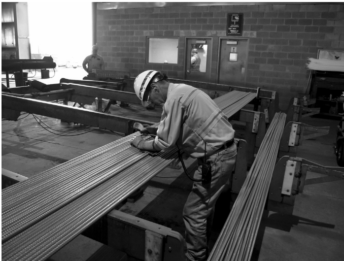
Figure 5.3 Measuring epoxy coating thickness as part of quality control within manufacturing.
