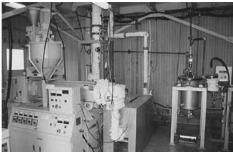
FIGURE 18.31 Plant for converting the PS waste to styrene monomer. (From Toshiba Co., Japan, 2006. With permission.)
