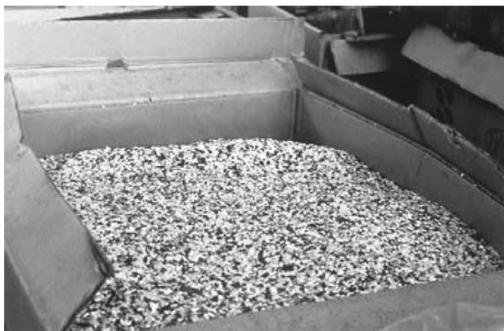
FIGURE 18.9 HDPE flakes separated from metal contamination by magnet. (From R. W. Beck, Inc., Seattle, WA, 2005. With permission.)
