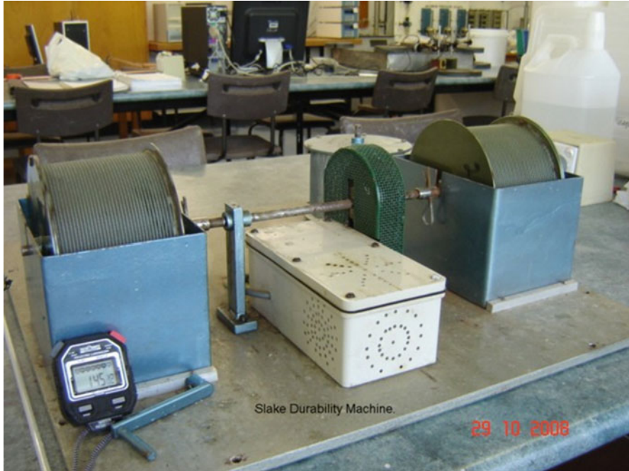
Fig. 9.3 Slake durability test apparatus
