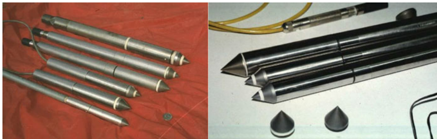
Fig. 5.2 Various Cone Penetrometers including Electric Friction and Piezocone types (After FHWA NHI-01-031 – Mayne et al. 2002)
