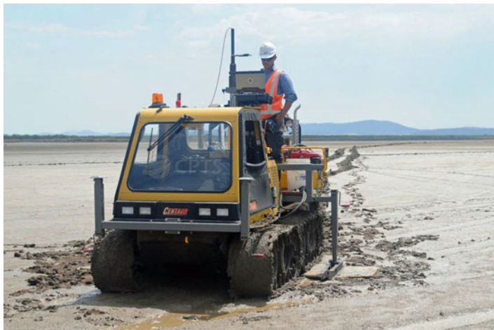
Fig. 5.1 CPT machine in mud flats (Courtesy Yvo Keulemans, CPTS)
