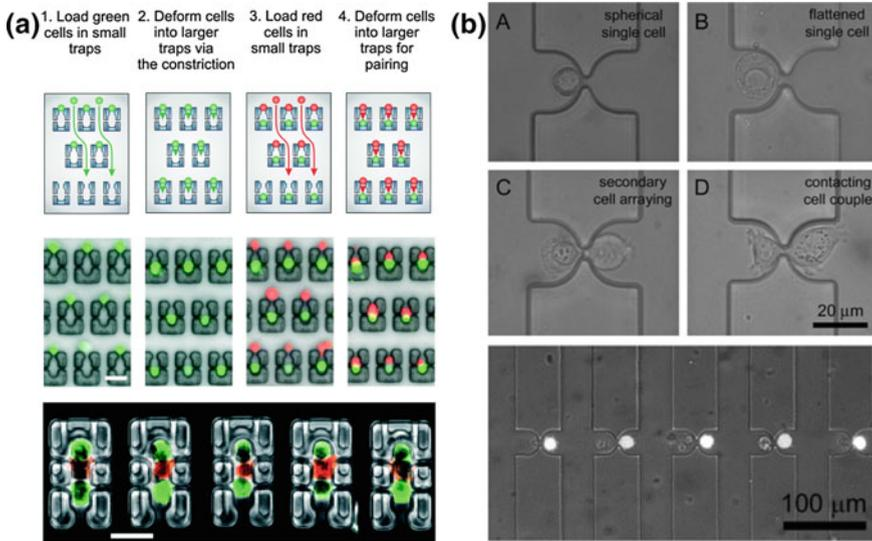
**Fig. 12** Examples of additional microfluidic platforms with potential applications for studying stem cell-niche cell interactions. Panel **a** Loading protocol for pairing cells into traps possessing lock-in features (*top*); two-component and three-component pairings demonstrated (*bottom*) [154]. Panel **b** Heterotypic single-cell co-culture arrays, pairing one unlabeled SW480 cell with one fluorescently labeled with calcein AM [155]
