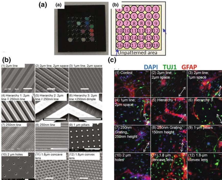
**Fig. 3** MARC chip for high-throughput topographical investigation of hESC neural differentiation. Panel **a** Schematic overview of chip design [72]. Panel **b** SEM images of single and multi-architectural PDMS patterns [72]. Panel **c** Immunostaining of hESCs for neuronal (Tuj-1 green) and astrocytic (GFAP, red) lineages on the different topographies [72]
