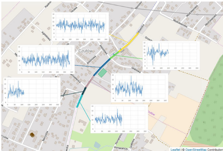
Fig. 3 Elementary road sections with linear accelerations assigned
