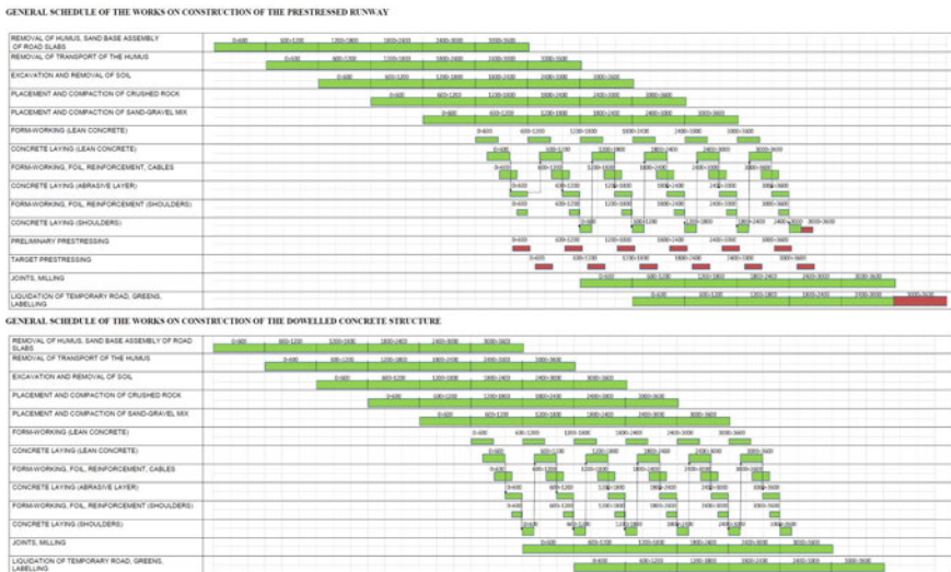
Fig. 2 General schedule of the works on construction of the prestressed runway and of the dowelled concrete structure
