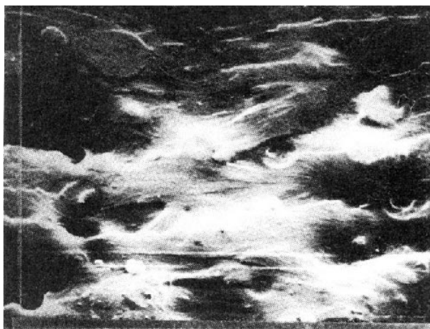
FIG. 45 SEM micrograph of fractured surface of PER/PBNCO 90/10 blend 0 (2500 \times ).
