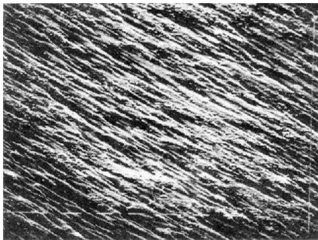
FIG. 42 SEM micrograph of fractured surface of plane PER resin (640 \times ).
