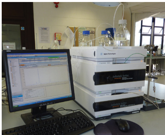
Figure 4.22 A typical laboratory HPLC system (a) and a selection of typical HPLC chromatographic columns (b).
