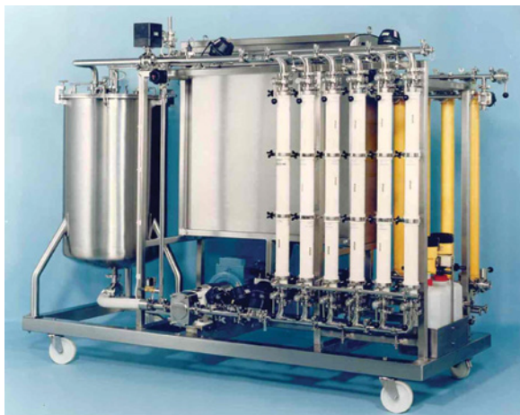
Figure 5.11 Example of an ultrafiltration system used on an industrial scale. This system (SPM 180) comprises 16.7 m 2 of spiral wound membrane. It can be used in ultrafiltration or diafiltration mode. Photograph courtesy of Amicon Ltd.
