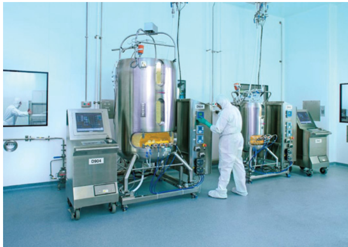
Figure 5.7 Typical bioprocess-scale fermentation equipment. Photo of a 20 litre pilot scale/small bioprocess-scale fermentation unit (a). Photo of a process scale mammalian cell culture facility, housing a 1000 litre bioreactor (on the left) and a 200 litre scale bioreactor (on the right), (b). Photo (b) copyright FUJIFILM Diosynth Biotechnologies UK Ltd, www.fujifilmdiosynth.com
