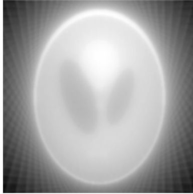
Fig. 3.4. The back projection of the Radon transform of the Shepp-Logan phantom.
