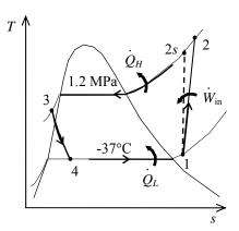
The actual enthalpy at the compressor exit is determined by using the compressor efficiency:
