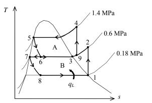
**11-121E** A two-evaporator compression refrigeration cycle with refrigerant-134a as the working fluid is considered. The cooling load of both evaporators per unit of flow through the compressor and the COP of the system are to be determined.
