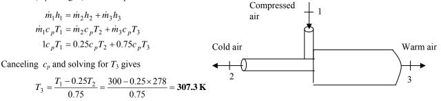
Therefore, the hot air stream will leave the vortex tube at an average temperature of 307.3 K.
