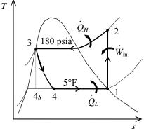
The mass flow rate of the refrigerant is
