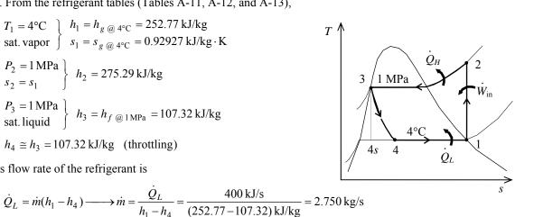
Assumptions 1 Steady operating conditions exist. 2 Kinetic and potential energy changes are negligible. Analysis In an ideal vapor-compression refrigeration cycle, the compression process is isentropic, the refrigerant enters the
