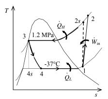
The actual enthalpy at the compressor exit is determined by using the compressor efficiency:
