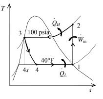
**11-46** A heat pump operating on the ideal vapor-compression refrigeration cycle with refrigerant-134a as the working fluid is considered. The COP and the rate of heat supplied to the evaporator are to be determined.
