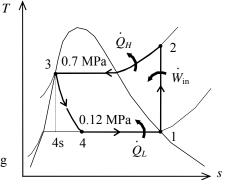
**11-17** A refrigerator with refrigerant-134a as the working fluid is considered. The rate of heat removal from the refrigerated space, the power input to the compressor, the isentropic efficiency of the compressor, and the COP of the refrigerator are to be determined.
