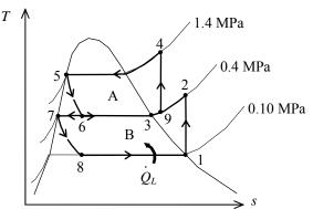
(b) The enthalpy at state 9 is determined from an energy balance on the mixing chamber:
