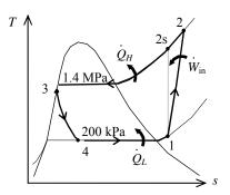
(b) Ideal vapor-compression refrigeration cycle solution From the refrigerant-134a tables (Tables A-11 through A-13)
