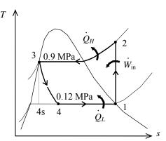
**11-16** An ideal vapor-compression refrigeration cycle with refrigerant-134a as the working fluid is considered. The throttling valve in the cycle is replaced by an isentropic turbine. The percentage increase in the COP and in the rate of heat removal from the refrigerated space due to this replacement are to be determined.
