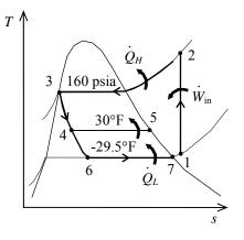
Application of this equation for each process of the cycle gives the exergy destructions per unit mass flowing through the compressor:
