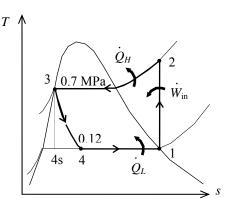
**11-15** An ideal vapor-compression refrigeration cycle with refrigerant-134a as the working fluid is considered. The rate of heat removal from the refrigerated space, the power input to the compressor, the rate of heat rejection to the environment, and the COP are to be determined.
