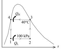
**11-4E** A steady-flow Carnot refrigeration cycle with refrigerant-134a as the working fluid is considered. The coefficient of performance, the quality at the beginning of the heat-absorption process, and the net work input are to be determined.
