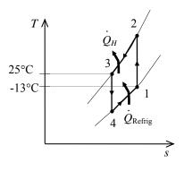
**11-80** A regenerative gas refrigeration cycle using air as the working fluid is considered. The effectiveness of the regenerator, the rate of heat removal from the refrigerated space, the COP of the cycle, and the refrigeration load and the COP if this system operated on the simple gas refrigeration cycle are to be determined.
