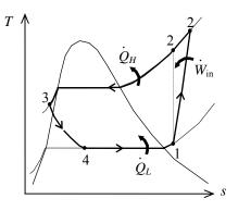
**11-21** A refrigerator with refrigerant-134a as the working fluid is considered. The power input to the compressor, the rate of heat removal from the refrigerated space, and the pressure drop and the rate of heat gain in the line between the evaporator and the compressor are to be determined.
