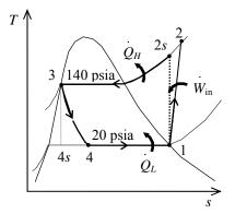
The energy interactions in each component and the mass flow rate of R-134a are
