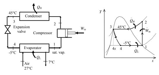
$$T_{1} = -5^{\circ}C \qquad h_{1} = h_{g@-5^{\circ}C} = 248.1 \text{ kJ/kg}$$
