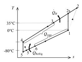
(*d*) The simple gas refrigeration cycle analysis is as follows:
