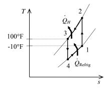
**11-78E** An gas refrigeration cycle with air as the working fluid has a compression ratio of 4. The COP of the cycle is to be determined.
