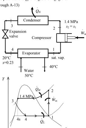
**11-50** An actual heat pump cycle with R-134a as the refrigerant is considered. The isentropic efficiency of the compressor, the rate of heat supplied to the heated room, the COP of the heat pump, and the COP and the rate of heat supplied to the heated room if this heat pump operated on the ideal vapor-compression cycle between the same pressure limits are to be determined.
