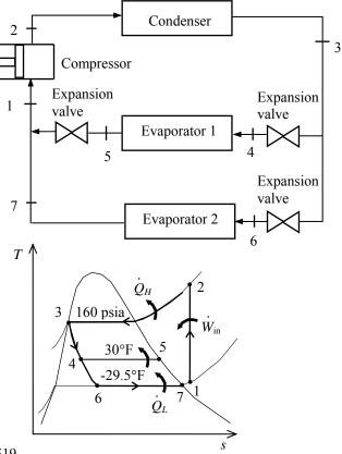
**11-122E** A two-evaporator compression refrigeration cycle with refrigerant-134a as the working fluid is considered. The process with the greatest exergy destruction is to be determined.
