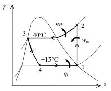
**11-26** A vapor-compression refrigeration cycle with refrigerant-134a as the working fluid is considered. The rate of cooling, the power input, and the COP are to be determined. Also, the same parameters are to be determined if the cycle operated on the ideal vapor-compression refrigeration cycle between the same pressure limits.
