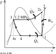
**11-35** An ideal vapor-compression refrigeration cycle is used to keep a space at a low temperature. The cooling load, the COP, the exergy destruction in each component, the total exergy destruction, and the second-law efficiency are to be determined.
