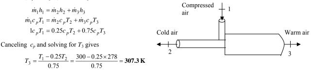
Therefore, the hot air stream will leave the vortex tube at an average temperature of 307.3 K.
