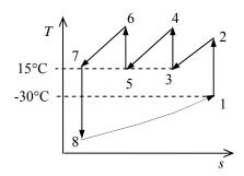
**11-132** A vortex tube receives compressed air at 500 kPa and 300 K, and supplies 25 percent of it as cold air and the rest as hot air. The COP of the vortex tube is to be compared to that of a reversed Brayton cycle for the same pressure ratio; the exit temperature of the hot fluid stream and the COP are to be determined; and it is to be shown if this process violates the second law.
