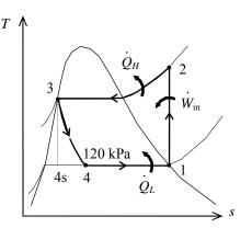
**11-24** A vapor-compression refrigeration cycle with refrigerant-22 as the working fluid is considered. The hardware and the T-s diagram for this air conditioner are to be sketched. The heat absorbed by the refrigerant, the work input to the compressor and the heat rejected in the condenser are to be determined.
