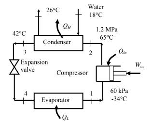
(b) The mass flow rate of the refrigerant may be determined from an energy balance on the compressor
