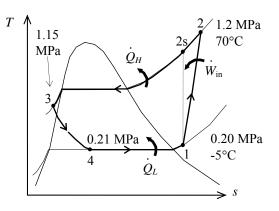
Then the rate of heat removal from the refrigerated space and the power input to the compressor are determined from
