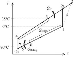
(c) The turbine and compressor powers and the COP of the cycle are
