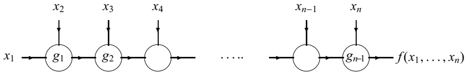
Figure 16. A sequence of circuits with Boolean functions g_1, g_2, \dots, g_n on a critical path P .
