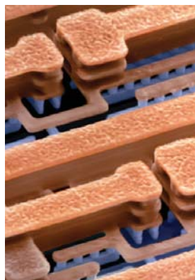
Figure 7. Microscopic view of a chip with copper-wiring (90 nm technology)
