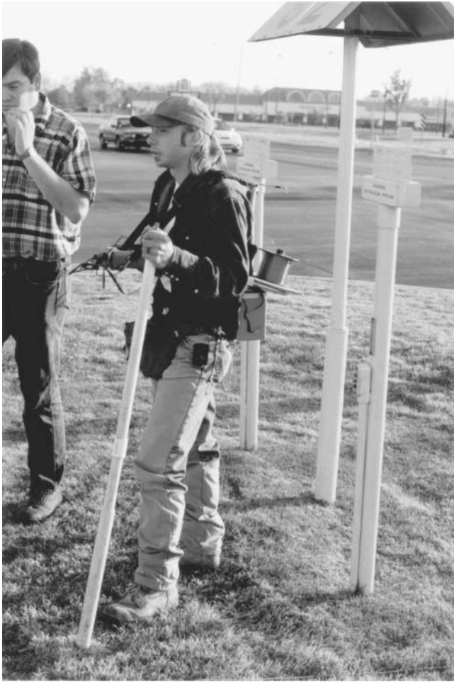
Figure 11.23 CIPS equipment, with the operator starting a survey at a test post. (Courtesy of CSIR North America Inc.)
