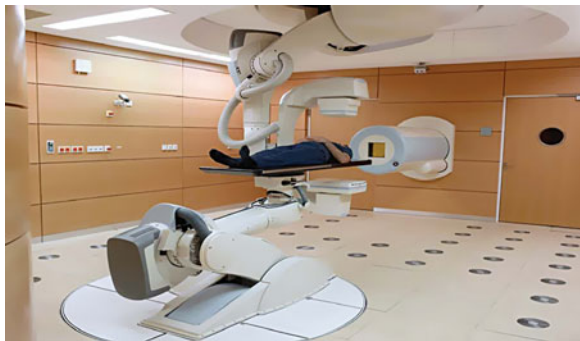
Fig. 29.8 The robotic imaging system installed in the treatment rooms at the Heidelberg Ion-Beam Therapy Center (HIT). The C-arm can be used for X-ray and fluoroscopic imaging in any direction, and is prepared for cone beam CT imaging
