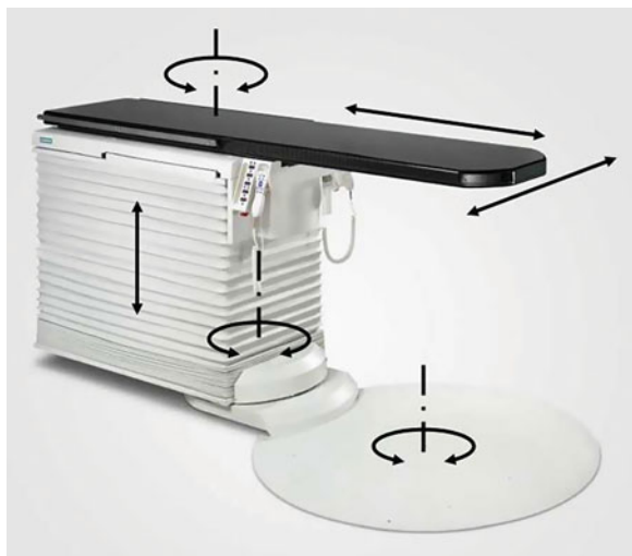
Fig. 33.1 Present-day treatment table for conventional RT with movement characteristics. The column rotation axis is used to move the table out of the isocenter. This axis is used for extended SSD (source-to-surface distance) treatments. Not all commercial tables share this feature though
