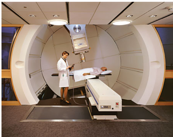
Fig. 35.2 View of a treatment room with gantry, including the beam delivery nozzle ( hanging from above ) and the patient positioning system (PPS)
