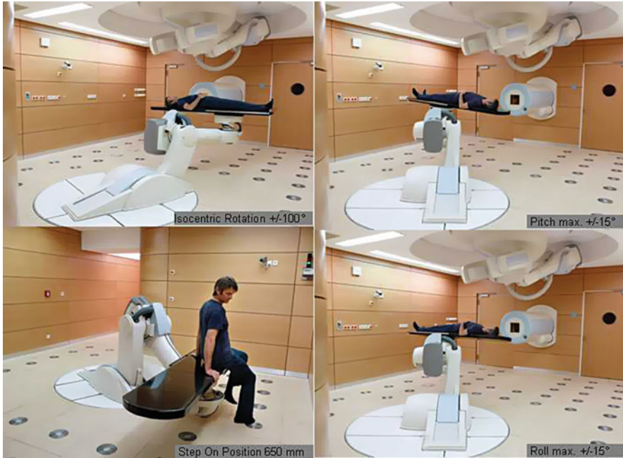
Fig. 33.9 Robotic patient positioner manufactured by Siemens for the Heidelberg Ion-Beam Therapy Center (HIT). Some of the possible positions typically used during patient treatment are shown
