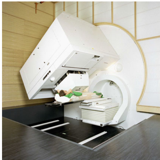
Fig. 24.1 Photograph of Gantry 1, the first proton scanning gantry of the world, which treats patients since 1996
