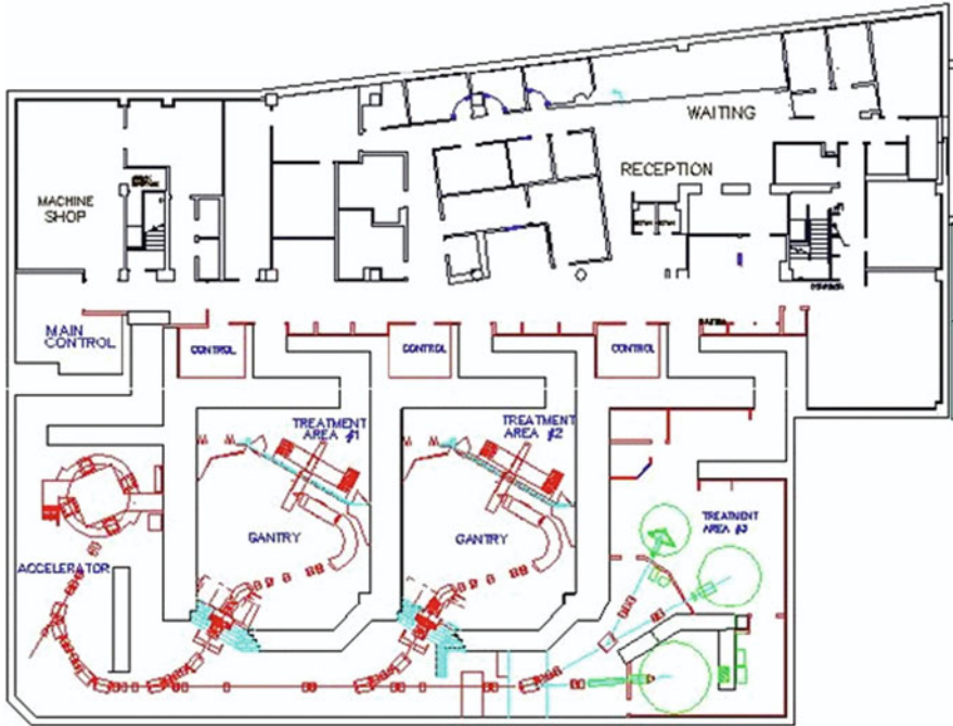
Fig. 35.5 Layout of the lower level of the FHBPTC including clinical rooms and most of the treatment equipment
