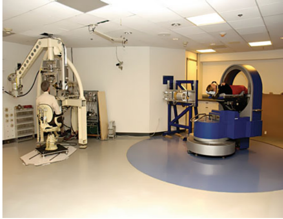
Fig. 35.3 Treatment equipment in the fixed-field room of the FHBPTC moved from the Harvard Cyclotron Laboratory (HCL). Left: Eye treatment station; Right: STAR (Stereotactic Radiation) positioner
