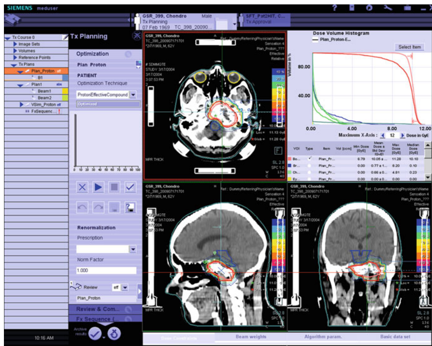
Fig. 8.7 View of the treatment planning system syngo TM PT planning by Siemens, Erlangen that uses the LEM to biologically optimize carbon ion treatment plans. Courtesy of HIT, Heidelberg
