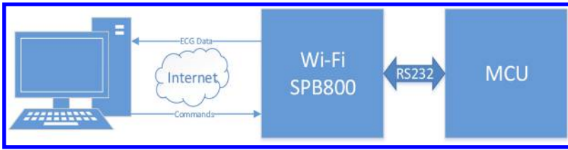
Figure 4. Basic Wi-Fi connectivity block diagram.
