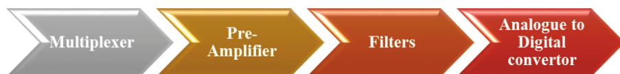
Figure 1. Block diagram of a conventional ECG system demonstrating the process of flow.
