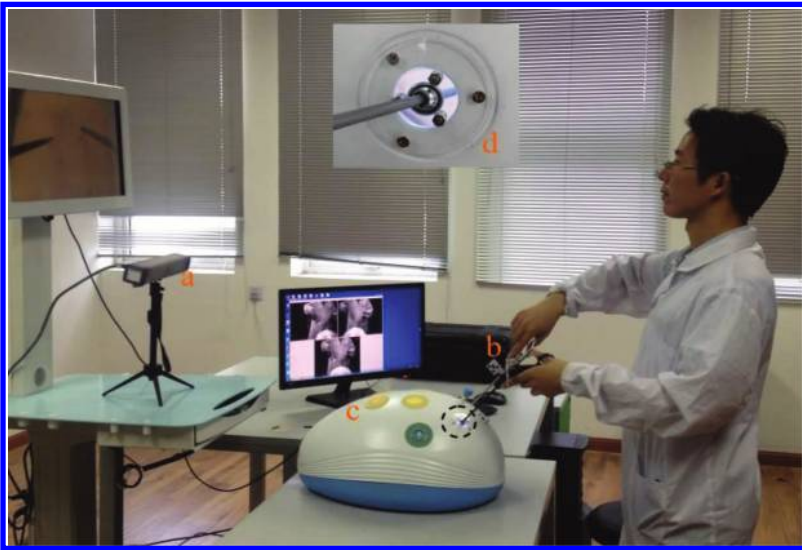
Figure 1. Experimental setup: (a) Tracking system. (b) Instrument with tracking marks. (c) Laparoscopic simulator. (d) Universal bearing for instrument insertion.
