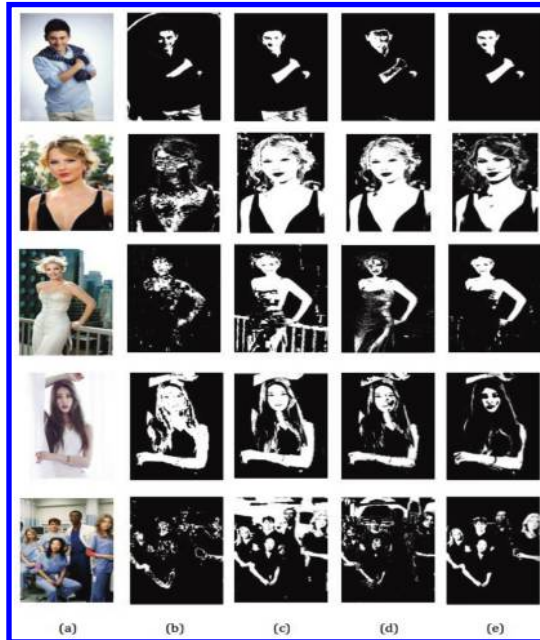
Figure 4. (a) Original Image. (b) 2-D histogram's result. (c) Gaussian model's result. (d) Dynamic threshold's result. (e) Fusion approach's result.
