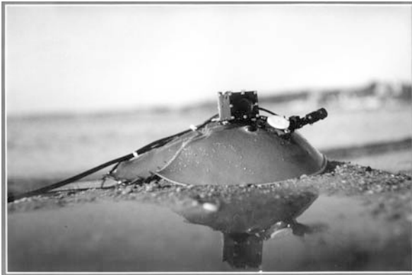
Fig. 3 A mini-video camera, CrabCam, mounted on an adult horseshoe crab records what the right lateral eye sees. A recording chamber mounted anterior to the eye contains a micro suction electrode (black cylinder on right) that records the response of a single optic nerve fiber through a whole drilled in the carapace. A white cap seals the recording chamber. The waterproof electrode and camera simultaneously record a nerve fiber's activity and the eye's underwater view as the crab searches for mates
