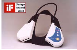
Fig. 2 Energy expenditure measurement system
