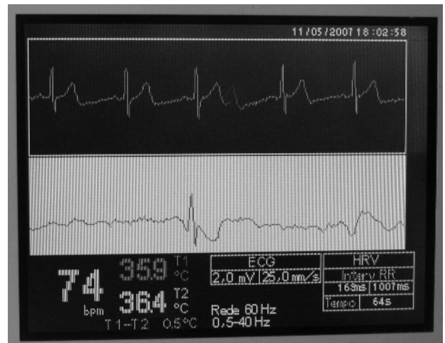
Fig. 4 CP CLCD showing the signals coming from FE and tachogram
