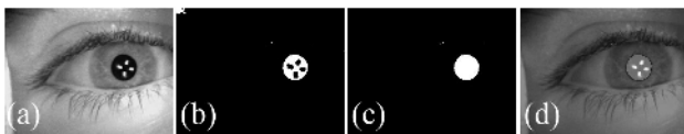
Fig. 4 Images obtained during automatic pupil radius determination. (a) Original, (b) binarized, (c) after morphological processing, and (d) images (a) and (c) combined.
