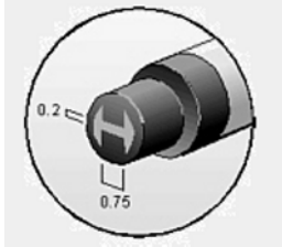
Figure 2: Detailed view of the „flush-mounted“ hot-film probe head.
