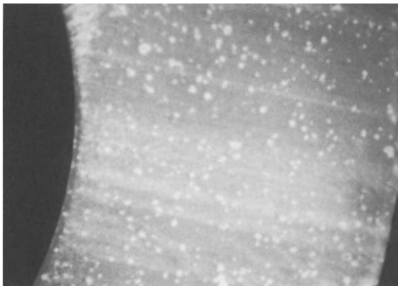
FIG. 2. This 200- \mu\text{m} slice of polyethylene shows the so-called fusion defects, also known as unconsolidated polyethylene particles
