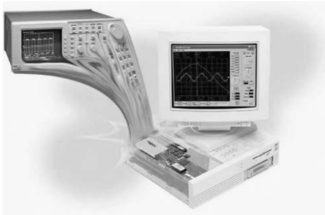
Figure 5.5-1 VI: Replicating and enhancing traditional “vendor-defined” instruments with virtual “user-defined” instruments. (Courtesy of National Instruments.)
