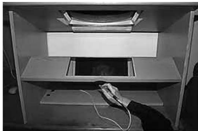
Figure 6.6-15 Virtual workbench. (Left) Schematic diagram illustrating the concept of reach-in work space. (Right) Prototype model of the workbench. (Photos courtesy of Timothy Poston, Luis Serra.)
