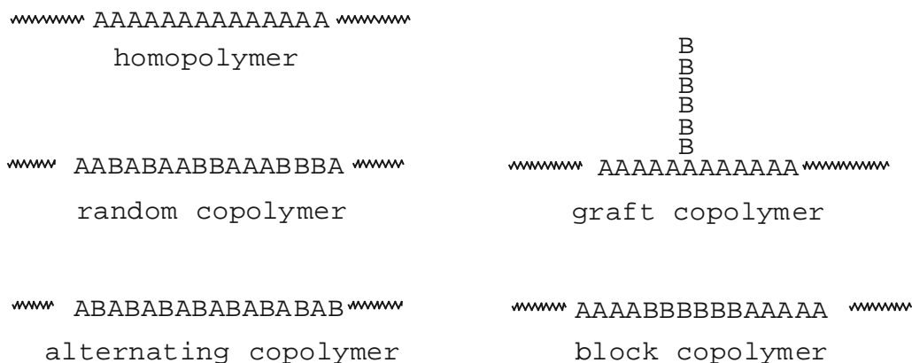
Fig. 3.2.2-4 Possible structures of polymer chains.
