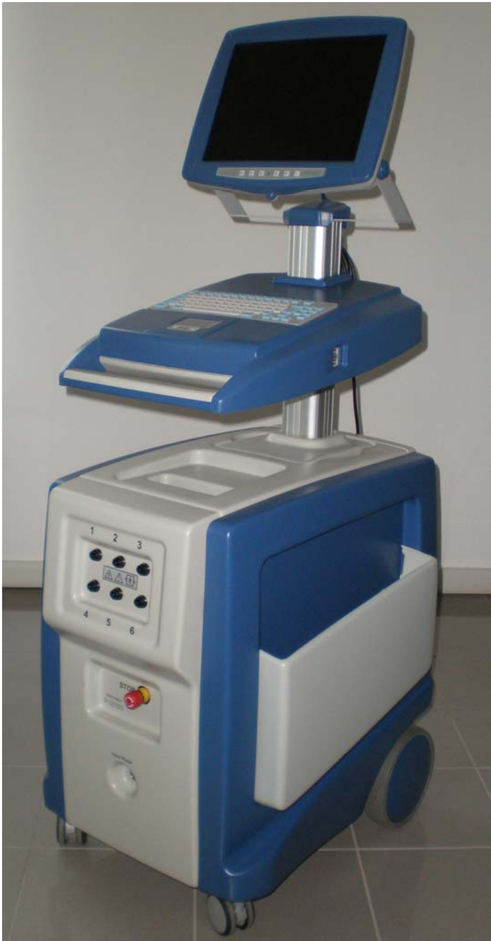
Fig. 7. Trolley containing the high voltage power unit at the bottom and the PC with the user interface (keyboard, touchpad and display) on top
