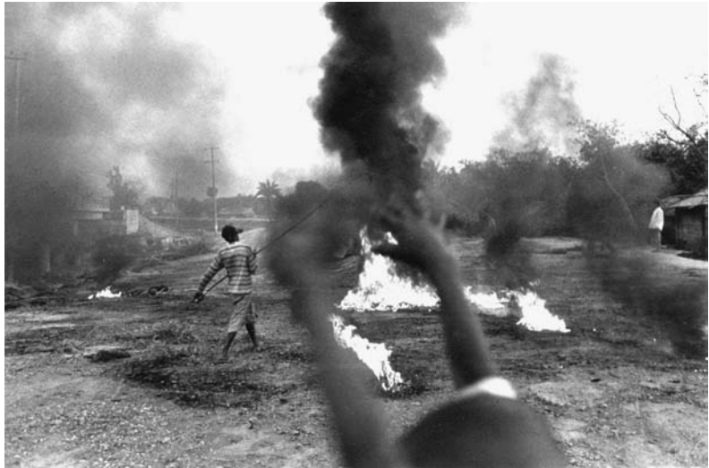
Figure 11.7 Shipbreakers burning rubber casing of copper wire in Chittagong, Bangladesh. Credit: Claudio Cambon, Marina Del Rey, California (Copyright, 1998)
