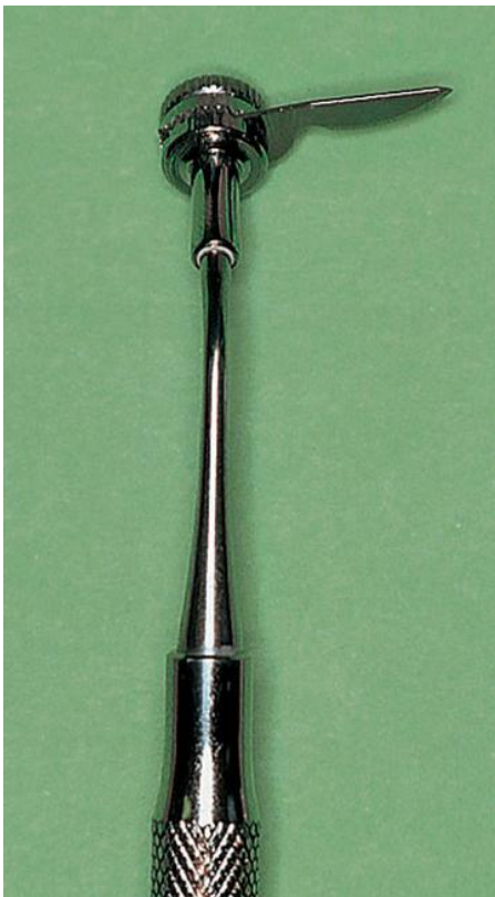
Fig. 39-47 Universal 360° handle for disposable blades, which allows the mounting of the blade in any angulated position of choice.
