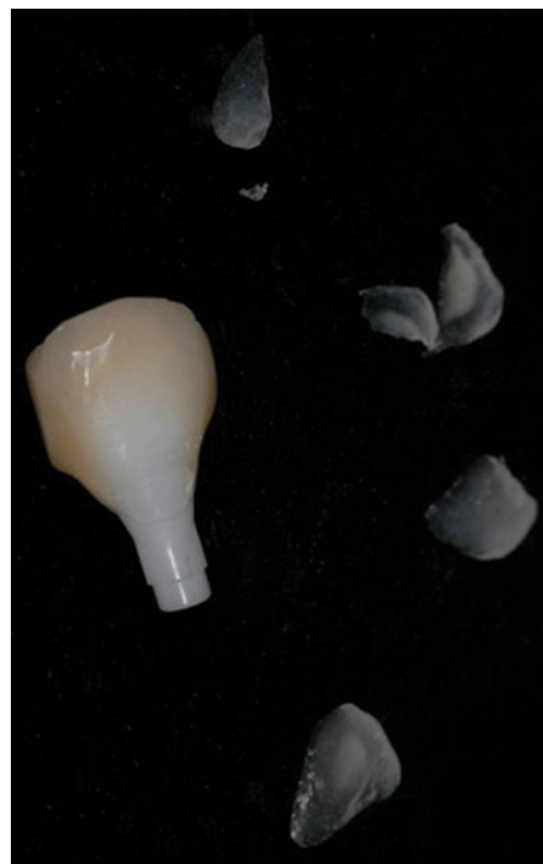
Fig. 55-46 Fractures of the cervical portion of the veneering ceramic (chips) at a posterior single-tooth zirconia-based crown.
