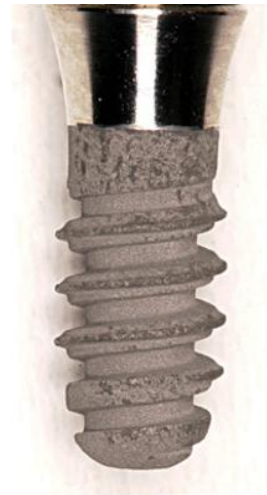
Fig. 5-10 Device used in the dog experiment. The implant is a modification of a solid screw (Straumann® Implant System). The distance between two consecutive threads is 1.25 mm. The depth of the trough is 0.4 mm. (Courtesy of AstraTech.)
