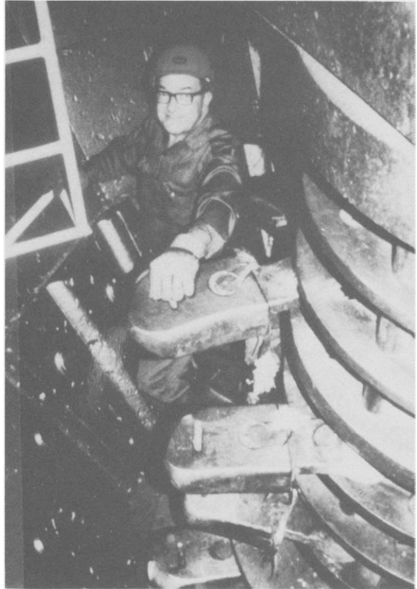
FIGURE 14-3 Inside a vertical hammermill. The hammers have been worn down by the shredding process. [Courtesy W. A. Worrell.]
