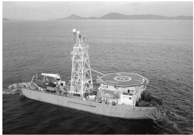
FIGURE 109 Vessels for offshore CPTs: ( left ) Markab, Australia; ( right ) Bucentaur, Brasil (Courtesy: Fugro Geosciences).
