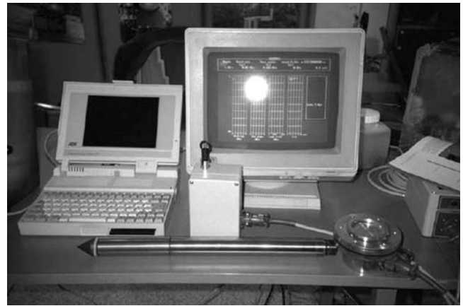
FIGURE 89 Cableless CPT systems: (left) Memocone (ENVI) and (right) audio-signal unit (Geotech AB).
