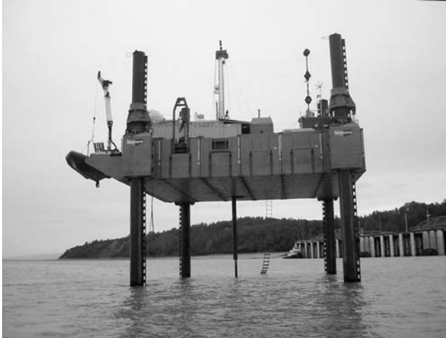
FIGURE 108 Jackup rigs for nearshore CPT deployment: ( left ) SeaCore, and ( right ) The Explorer.
