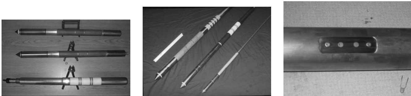
FIGURE 87 Electrical conductivity measurements: ( left ) Fugro conductivity cones, ( center ) Vertek Dielectric and Hogentogler resistivity cones, and ( right ) Diametric (Button) Electrode Array for Resisitivity.
