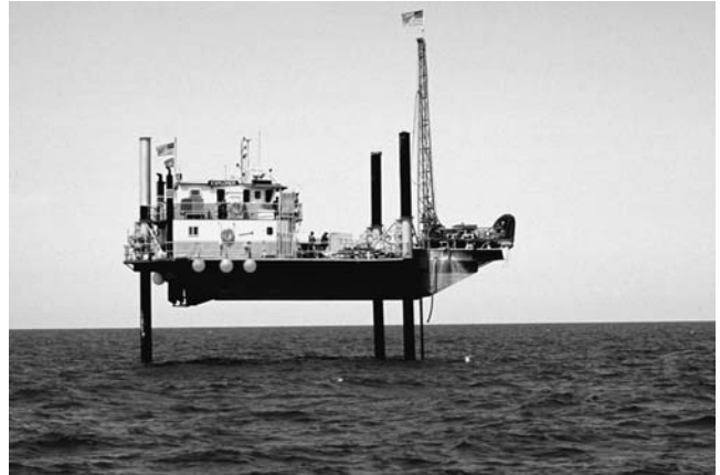
FIGURE 108 Jackup rigs for nearshore CPT deployment: ( left ) SeaCore, and ( right ) The Explorer.
