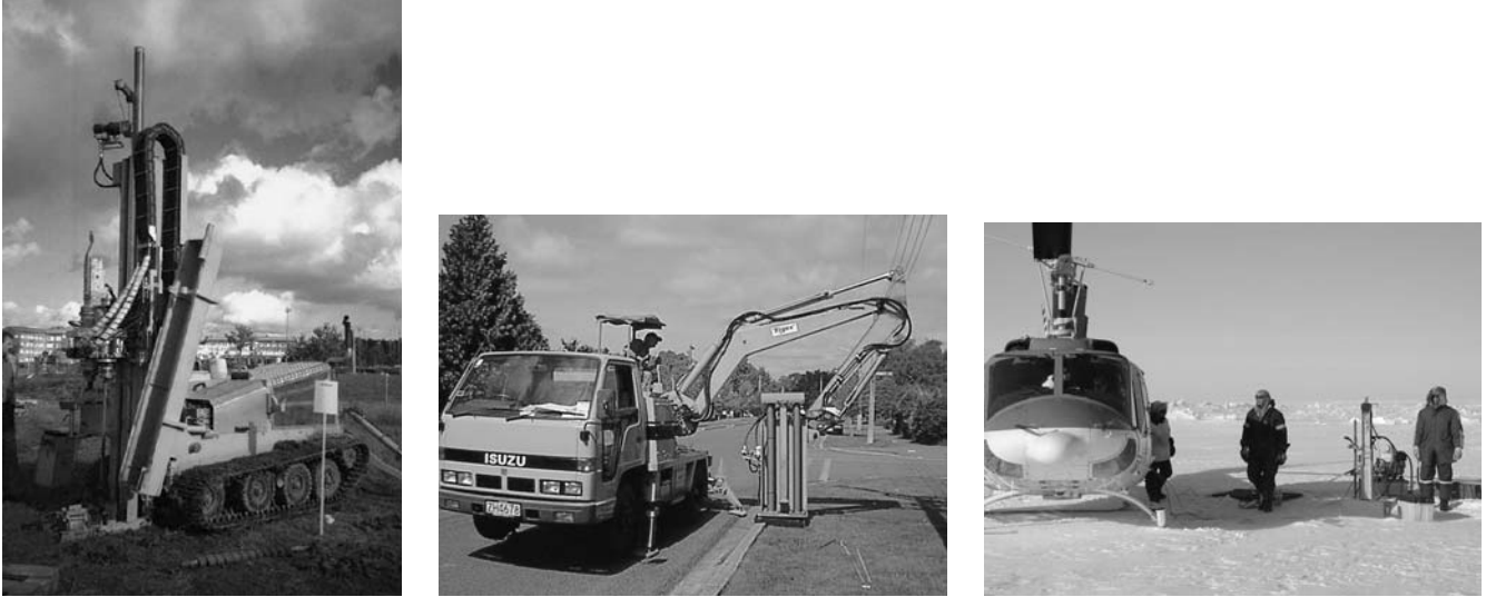
FIGURE 96 Special CPT deployment systems: ( left ) single personnel track vehicle (Sweden), ( center ) cherry-picker for urban access (New Zealand), and ( right ) portable unit for arctic work (Canada).
