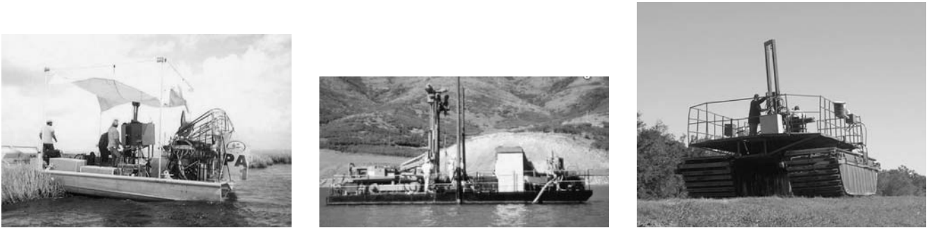
FIGURE 97 Special CPT deployment by ( left ) airboat, ( center ) barge, and ( right ) New Orleans marsh buggy.
