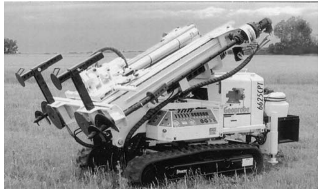
FIGURE 100 CPT vehicles for hard ground including: (left) 40-ton truck, (right) anchored track rig.
