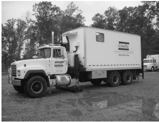
FIGURE 95 Rig with mounted hydraulic autoseis unit for deep downhole testing.
