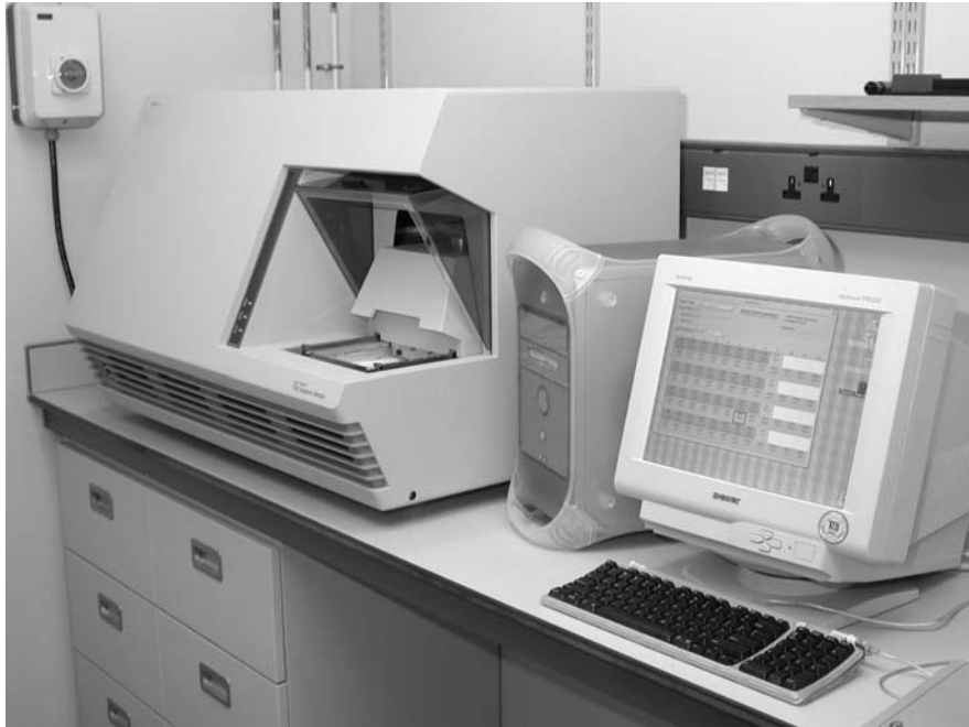
Figure 2.6 An ABI 7700 quantitative PCR machine (photograph courtesy of David Bacon, Imperial College, London)
